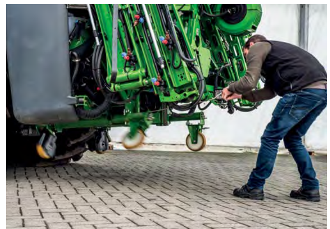
✓ Swivelling in and out the parking device
