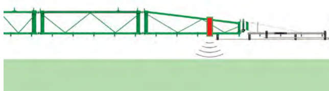
DistanceControl when equipped with two sensors: measuring to the crop
