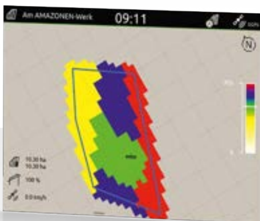
Display of the application map in AmaTron 4
