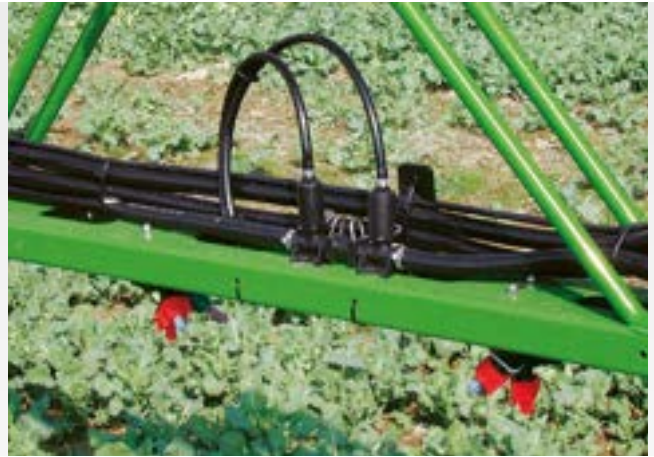
DUS pressure recirculation system
