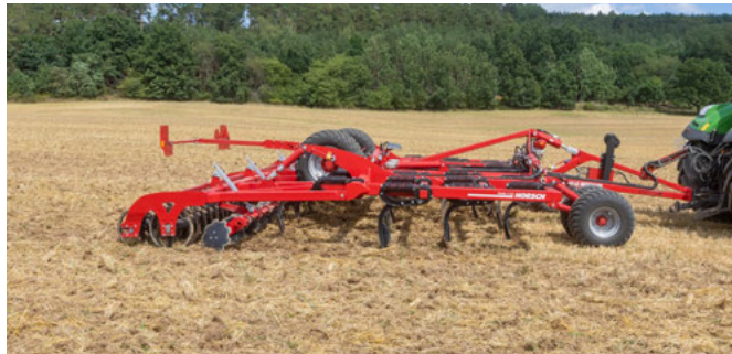
Rigid packer frame with double packer
