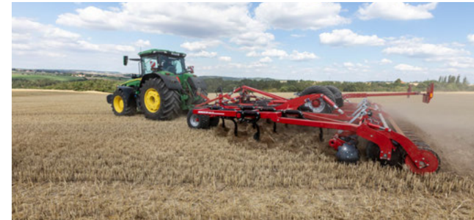
SteelFlex packer with hydraulically pre-tensioned RingFlex
