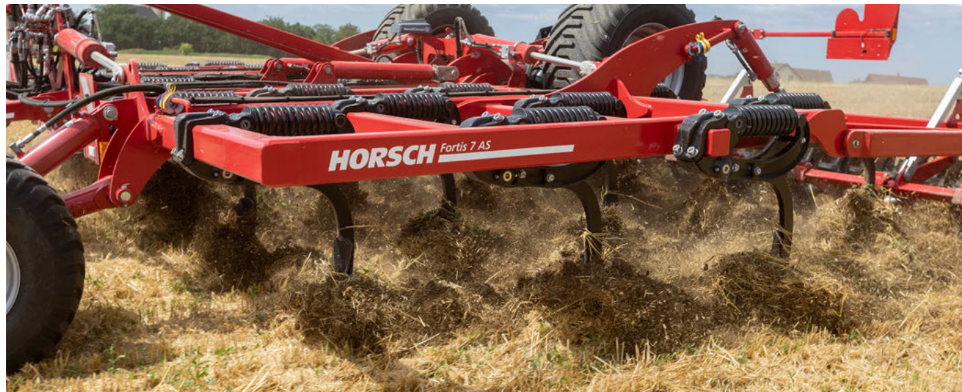
Excellent straw distribution as the straw remains in the tine system for a long time
