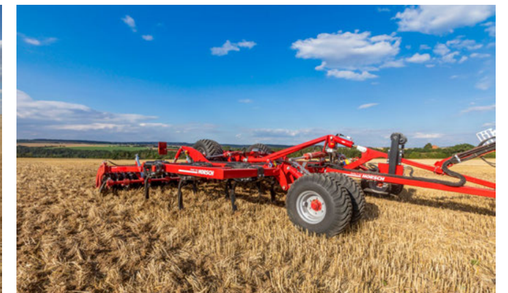
Front support wheels for even depth control
