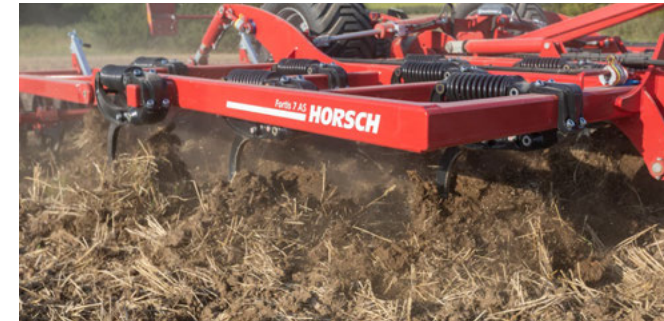
4-bar design for intensive mixing
