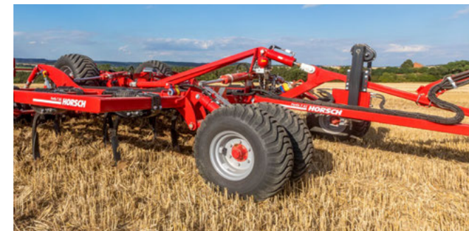
Front support wheels for even depth control
