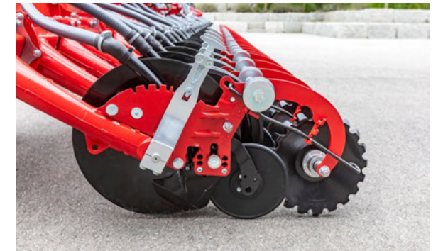
Steel star roller – produces fine soil and closes the seed furrow
