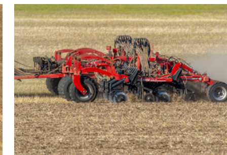
Smooth and directed hose routings ensure consistent flow of product at each opener.
