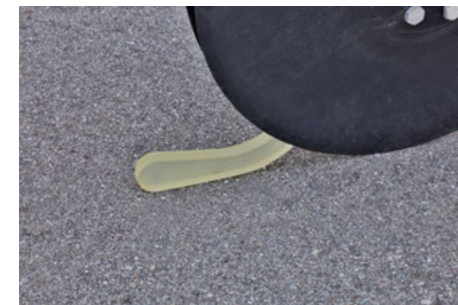
The HORSCH Uniformer ensures a precise embedment of the seed
