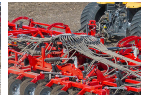
Straight seed towers and hoes for an even distribution of seed and fertilizer
