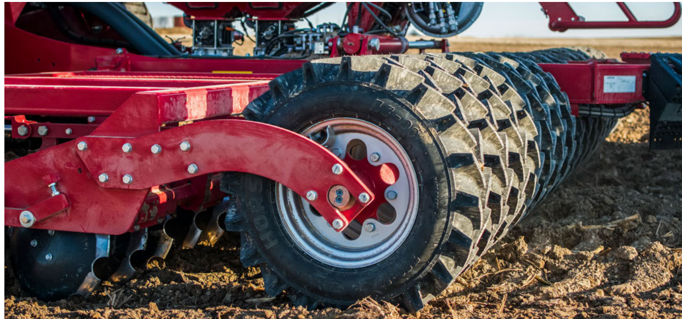
Front packer for better floatation and low horsepower requirement
