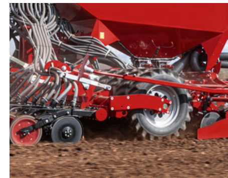
Efficient consolidation below the seed horizon for better retention of moisture in the seedbed
