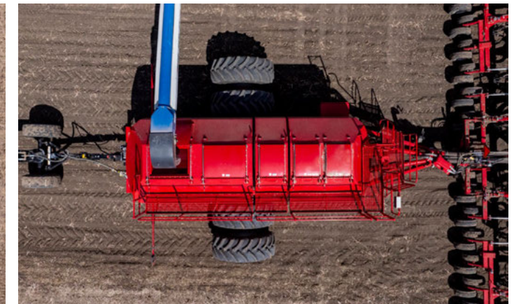
SW 600 features large hopper opening for easy filling
