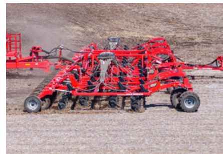
4-ranks of shanks and 15" shank spacing for no-till seeding
