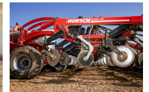
Unique 2-rank design provides narrow contour depth for precise seed placement in extreme variable field terrains
