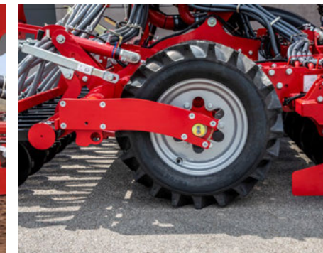
Low horsepower requirement due to large tire diameter and no scrapers required
