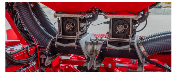
Double hopper S&F – meter different components separately and place them together in the furrow
