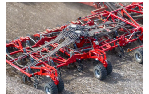
Big support wheels for precise seeding depth
