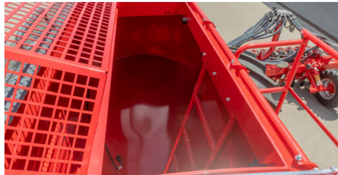
Hinged screens to prevent contaminations in the hopper
