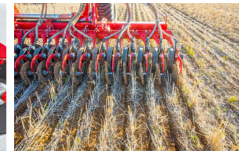
Low disturbance due to SingleDisc opener
