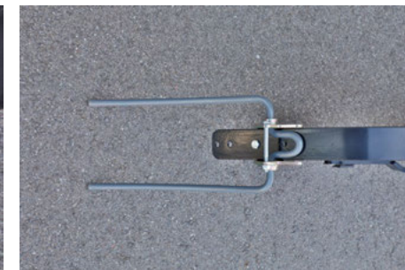
The straight harrow - TurboDisc opener harrow is controlled individually for a more efficient tillage
