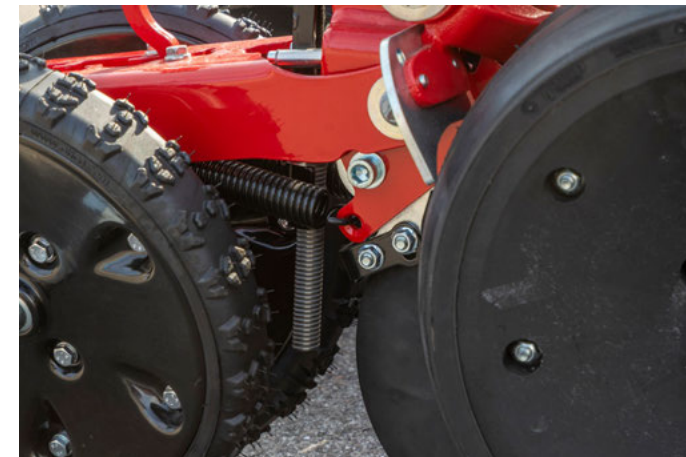
Liquid fertilizer application behind the catching roller
