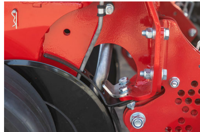
Liquid fertilizer application in the row
