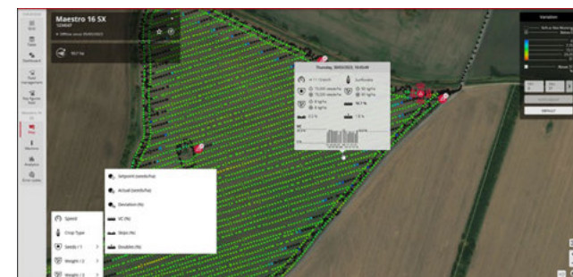
Success factor transparency: position-specific data of all relevant information like error messages, operational speed or singulation quality
