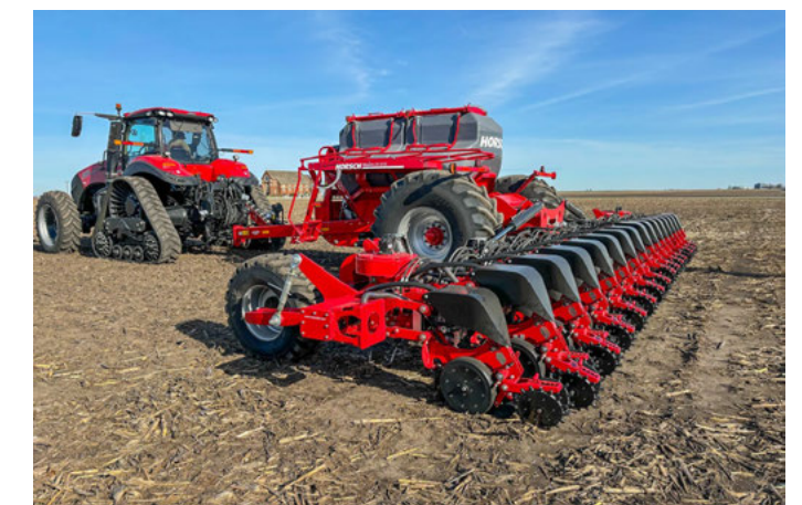
Maestro SV with 31 rows and 15’’ spacing
