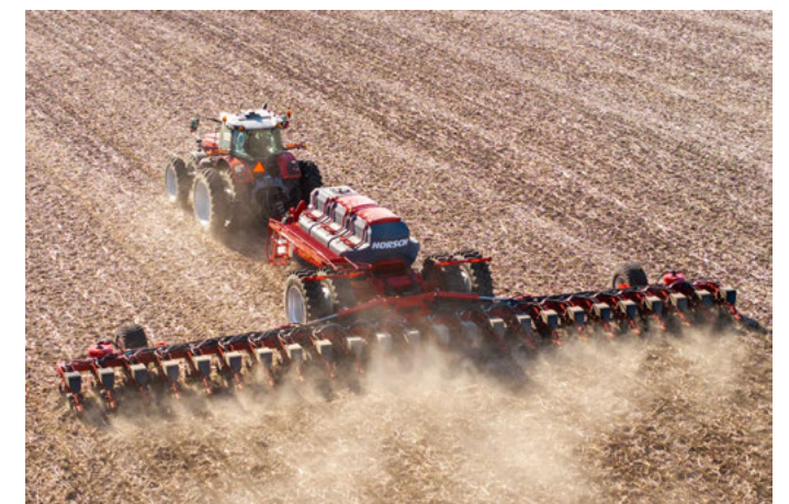
Maestro SV with 1230 gal of liquid fertilizer and 249 bu of seed capacity
