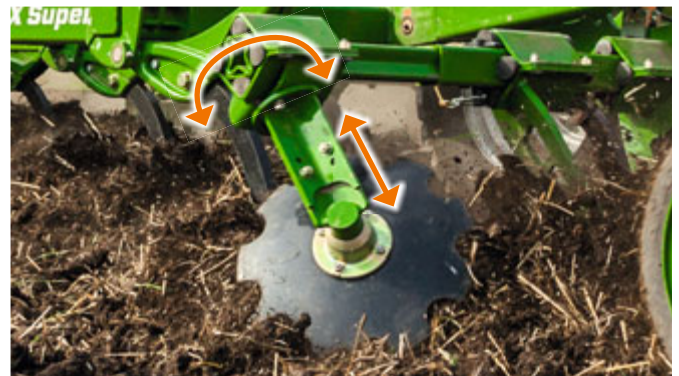
The outer closers – individually adjustable in height, angle, and position
