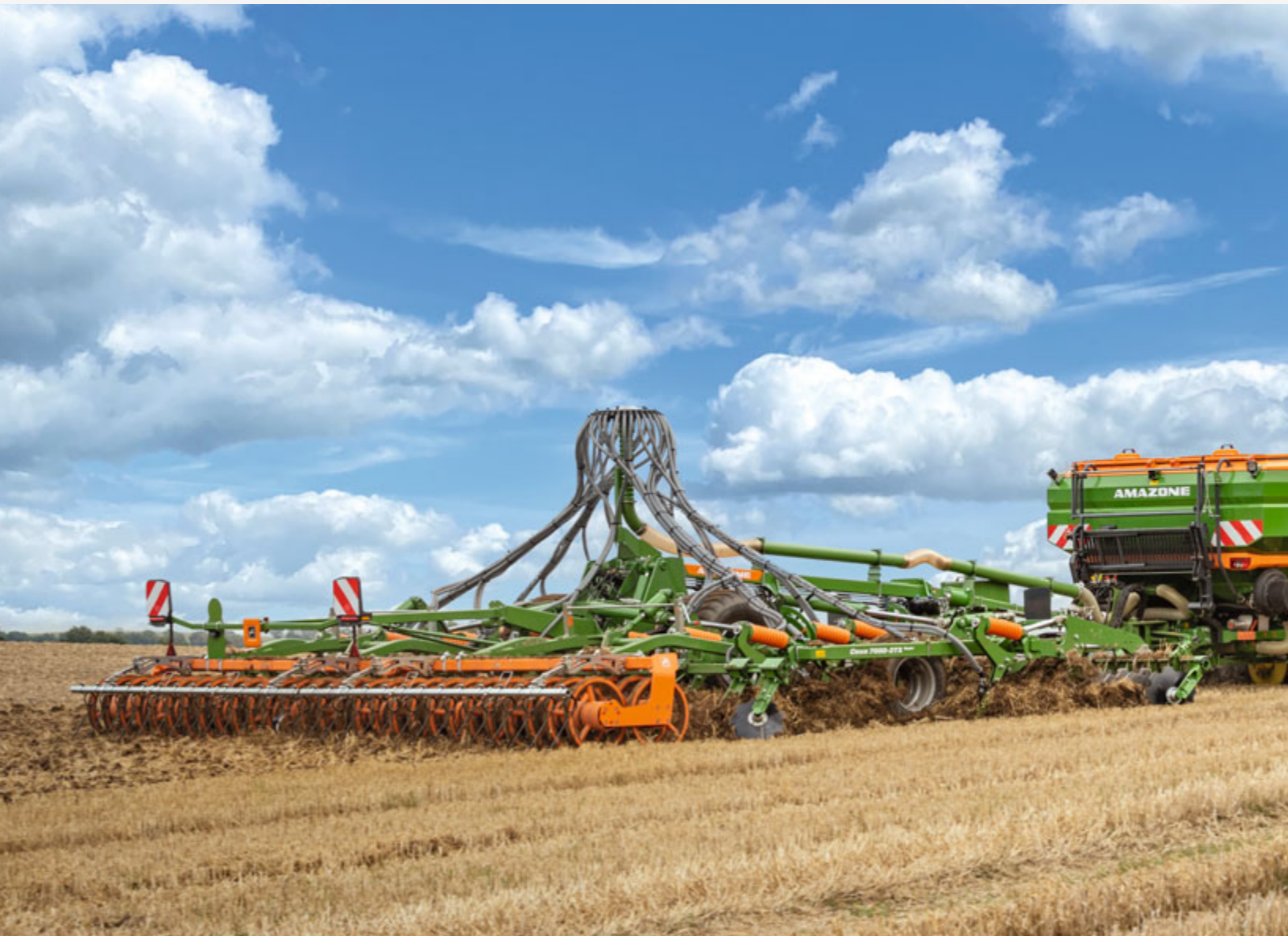
Ceus 7000-2TX Super combined with the XTender 4200 rear hopper for cover crop sowing or fertilization
