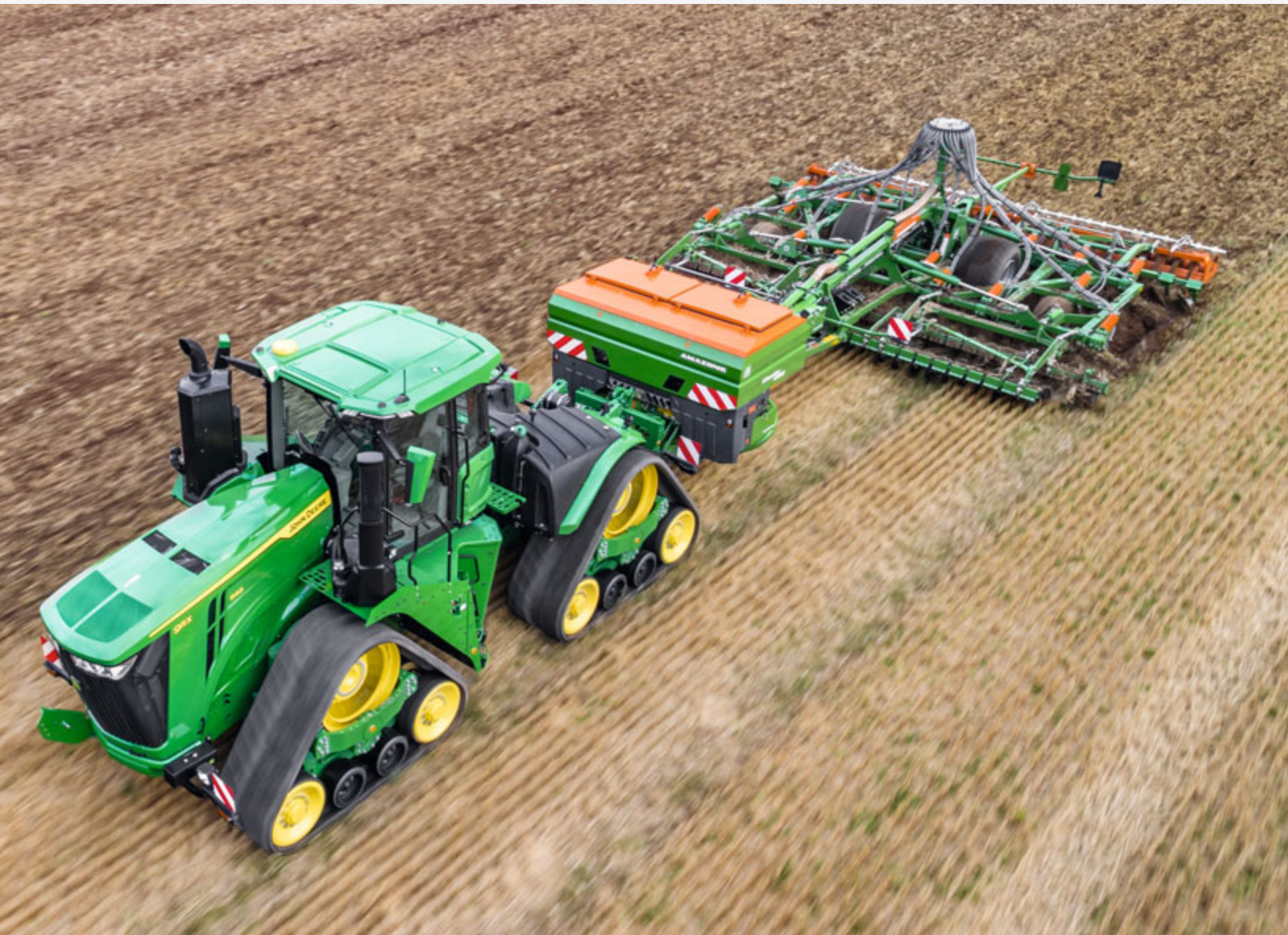
XTender 4200 with a capacity of 148 cu ft 120 bu (4,200 l)
