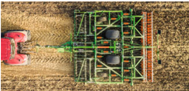
A tine behind each wheel loosens the wheel track
