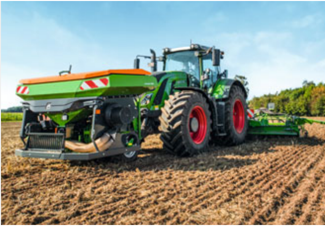
FTender 1600 mounted front hopper with a capacity of 56.5 cu ft 45.5 bu (1,600 l)
