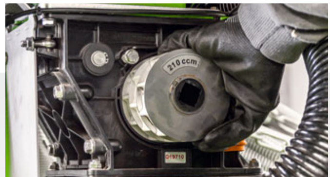
Easy exchange of the metering rollers
