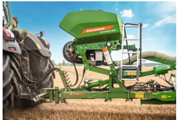
GreenDrill 501: for all trailed machines - with a 14.2 bu (500 l) hopper and hydraulic blower fan
