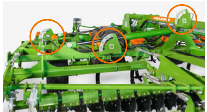
Working depth displays of the three tool implements all in one view
