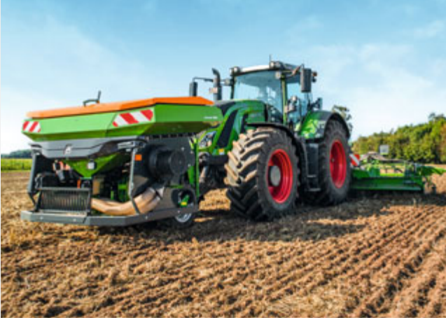
FTender 1600 mounted front hopper with a capacity of 45 bu (1,600 l)
