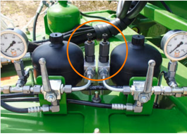
Standard drawbar damping system
