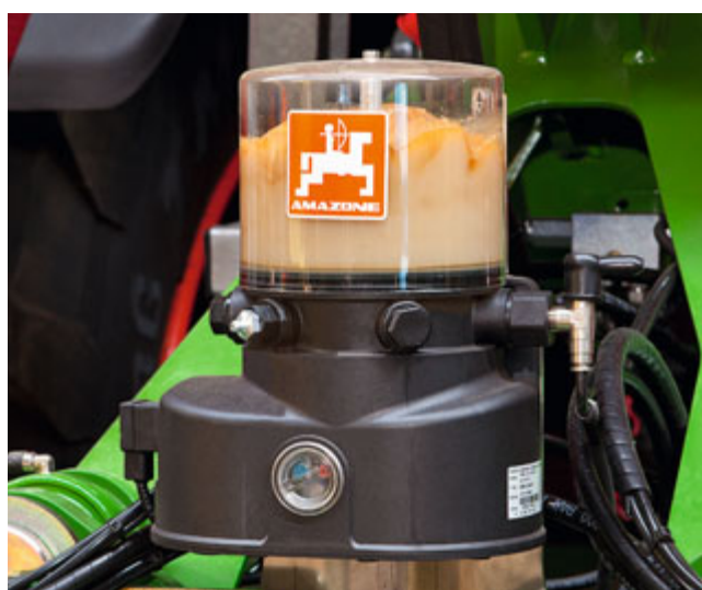
Pump with reservoir
