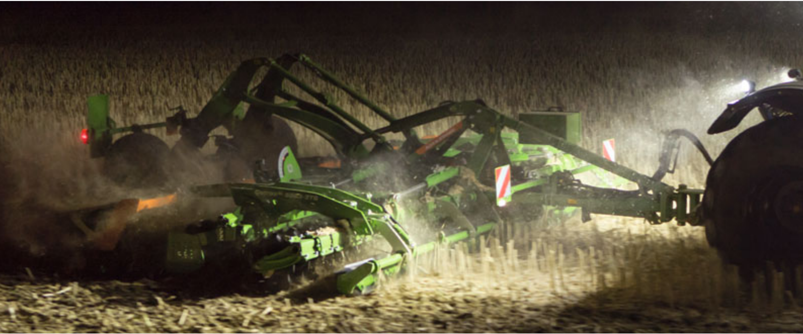
Catros XL with knife roller in canola stubble
