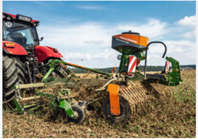
Catros XL 3003 with X-Cutter disc, knife roller and GreenDrill
