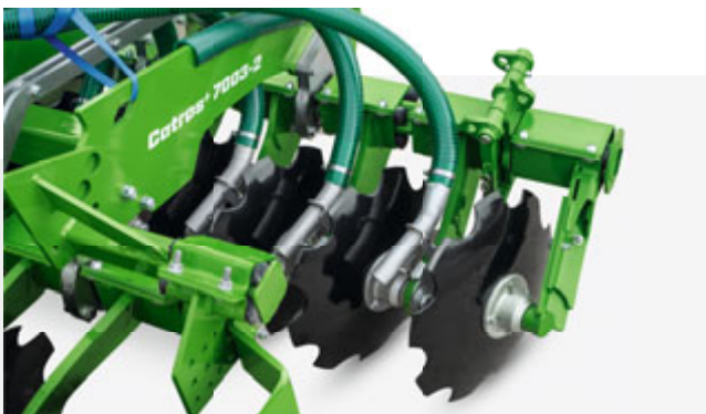
Slurry application after the first disc
