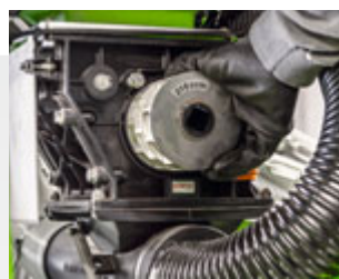
Easy exchange of the metering rollers
