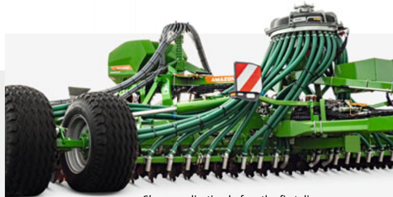
Slurry application before the first disc
