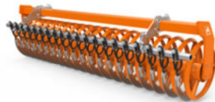
Spring-mounted knife system* for WW rear rollers
