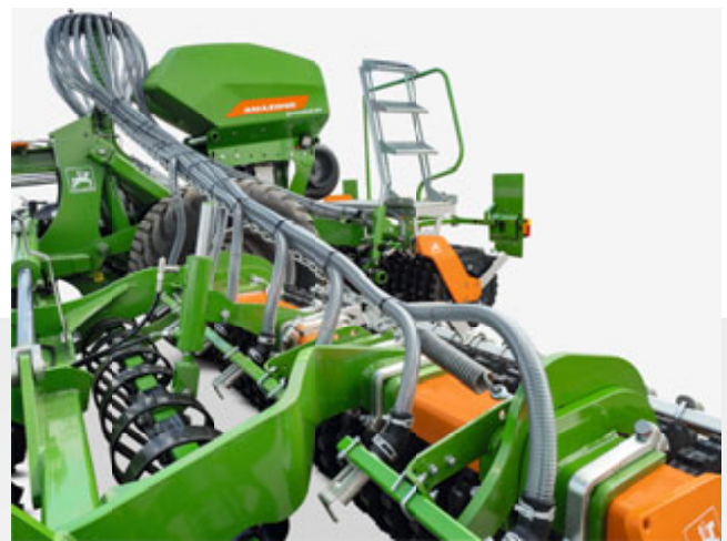
High flexibility provided by the segmented distributor head
