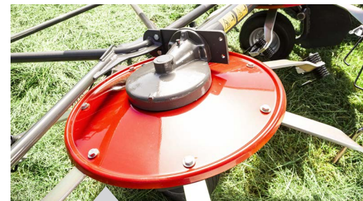
Large rotor diameter allows a high tine speed at a low rotor speed
