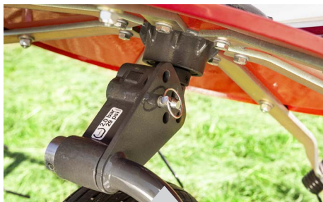
Five spreading angle settings are as easy to set as moving a pin, allowing you to precisely meet your needs
