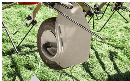
Anti-wrapping system prevents crop buildup around the wheel spindle
