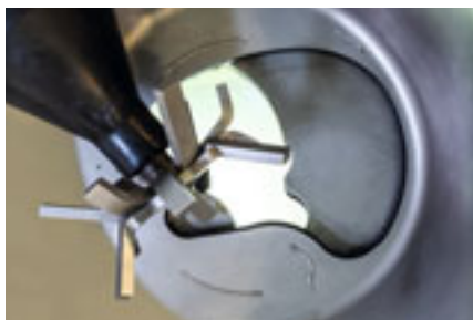
Stage 2: hopper shutter half open
