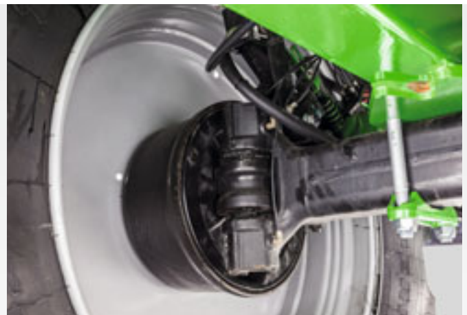
Braking force control via electronic braking system (EBS)
