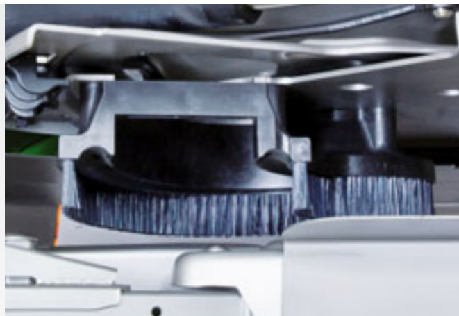
✔ Brush unit for a clean delivery onto the spreading discs
