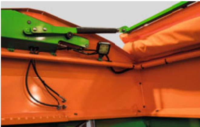
Work lights inside the hopper
