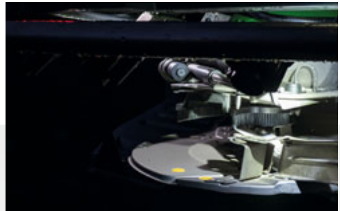
Illuminated spreading disc at night
