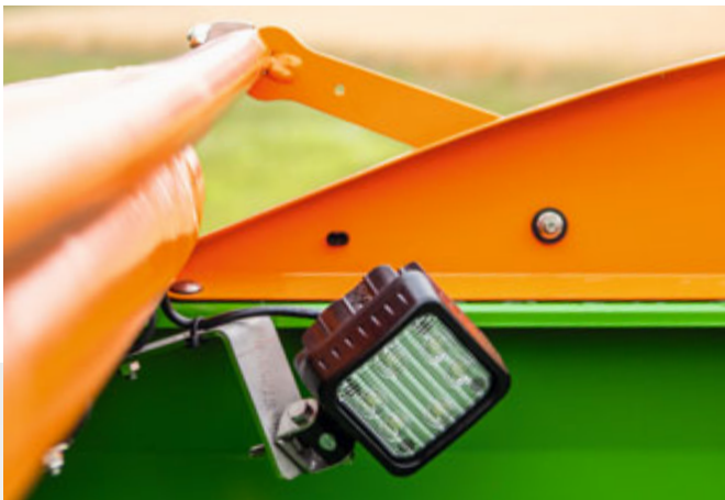
Lighting for the inside of the hopper
