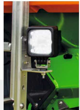
The steady beam of the work lights indicates that the pre-set full load capacity has been reached. the work lights
