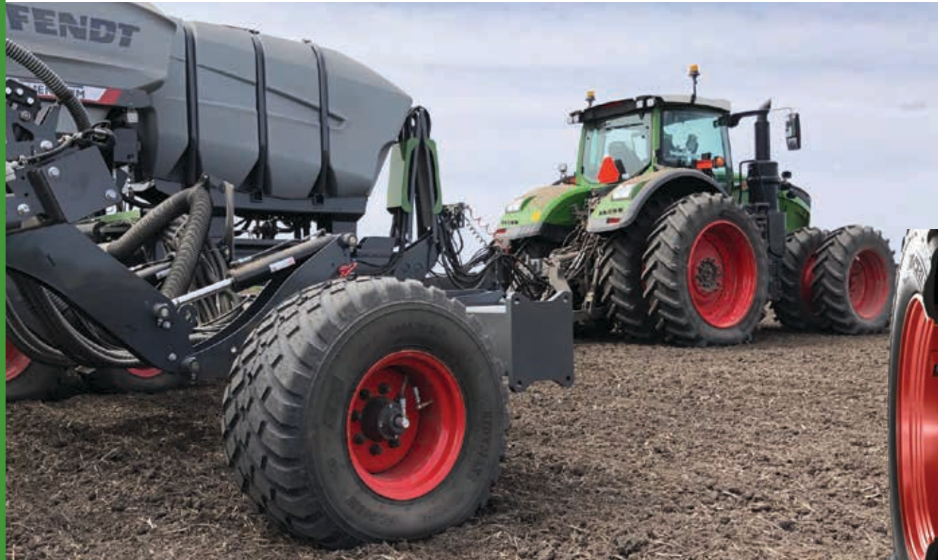
An onboard air compressor supplies air lines that are integrated into the wheel assembly. All components are secure and covered to prevent damage.
