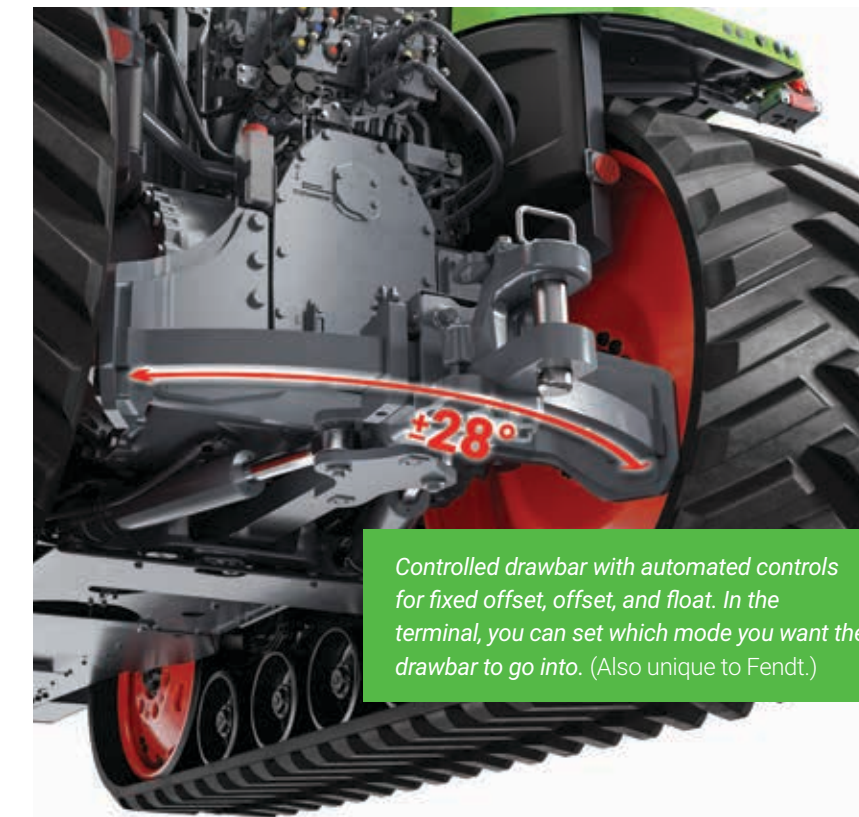
A new steerable hitch for mounted implements with automated controls unique to Fendt.
