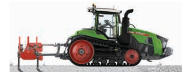
Figure 2: The 1100 Vario MT with Smart Ride Plus allows for easy adjustment of the weight distribution. This results in reduced slip, improved ride comfort, and improved overall performance.
