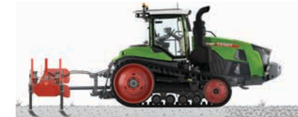
Figure 1: A tractor goes to work without proper tractor and implement weight distribution. This results in insufficient front weight on the tractor, and as a result increases slip.
