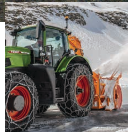
For applications that require a direct rear facing view, opt for the reversible driver's station. This innovative feature will pivot all cab elements 180 degrees for a direct rear view.
